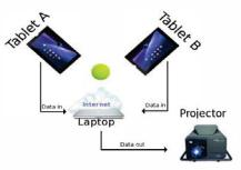
**Fig. 1.** Front-end system architecture of the TINB system. Two players play a game of paddle board with respective tablets. The data is relayed between the tablets and a third device, which can be connected to a projector to project the ball motion.
