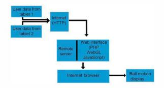
**Fig. 4.** Back-end system architecture of the TINB system. Data is filtered locally and transmitted to a remote server where calculations of the ball motion are carried out.
