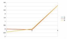
**Fig. 9.** Accelerometer values over time for swing of the tablet, transmitted to the server to calculate the ball motion.
